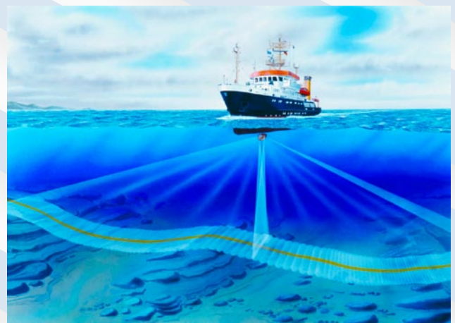
Fig 1. Multibeam echo sounders send out a sheet of sound either side of the ship.
